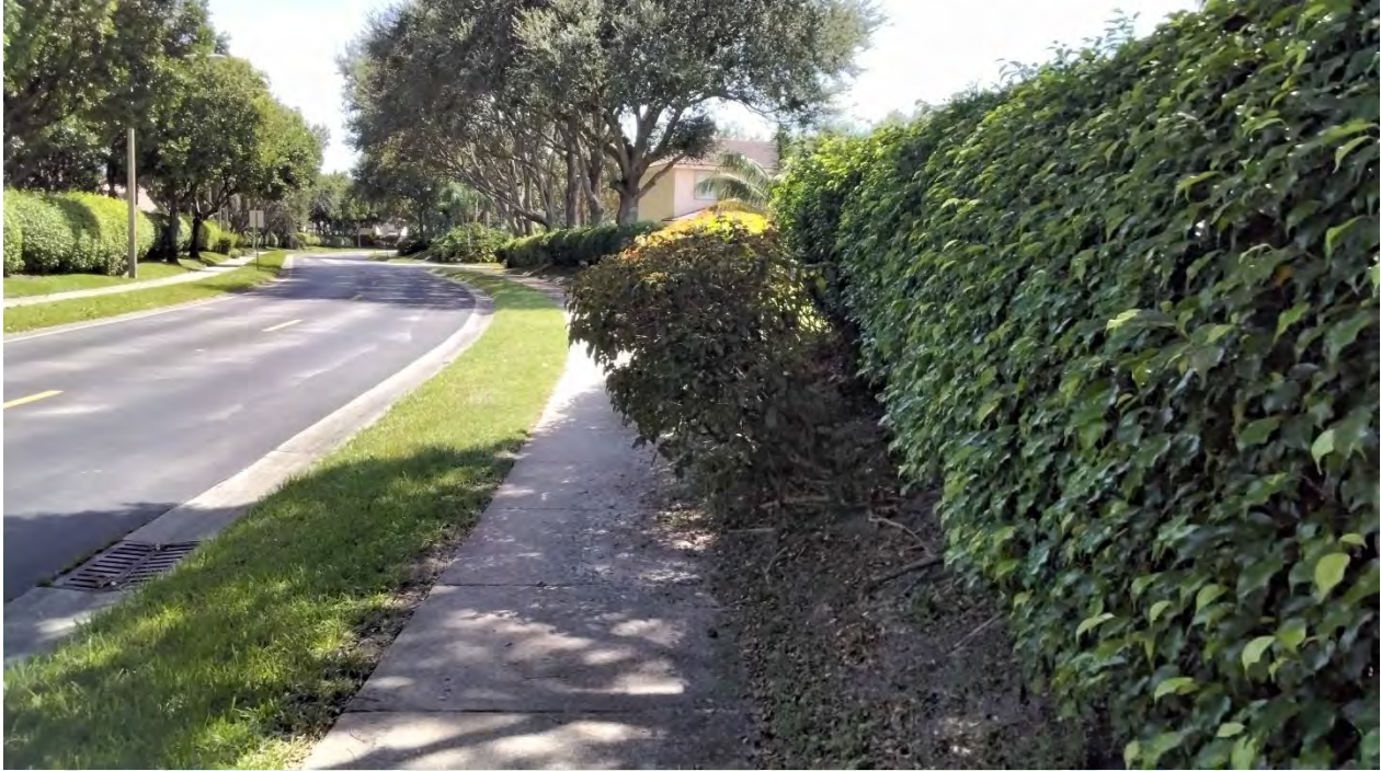
Above: Located along NW 76 th Ave. near the guard house. A hedge is growing over and onto the walkway. Pruning enough to provide ADA clearance will remove majority of foliage and branches. This hedge is in poor location next to the walkway, was not planted with adequate growing space, and now is pedestrian hazard. Removal is recommended, with groundcover or small maturing shrubs as replacement for first tier border between sidewalk and Ficus hedge..
